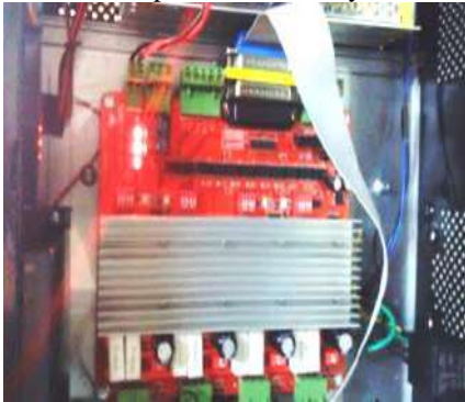
Figura 6. Tarjeta de control TB65603V2
